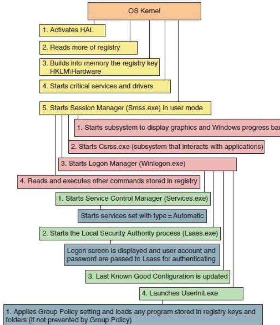
**Figure 6-22** Steps to complete loading Vista
