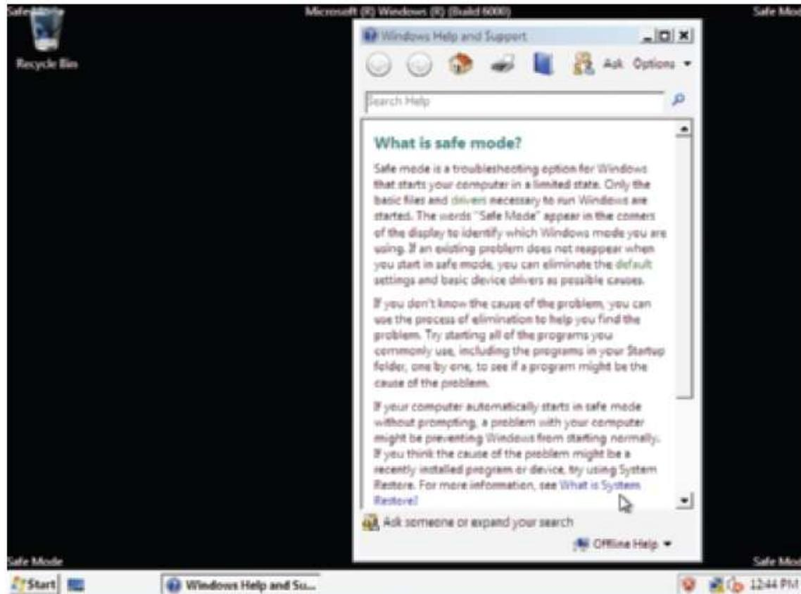
**Figure 6-28** Safe Mode loads a minimum Vista configuration
