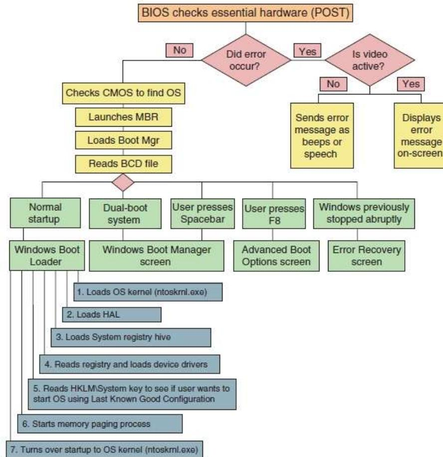
**Figure 6-21** Steps to booting the computer and loading Vista
