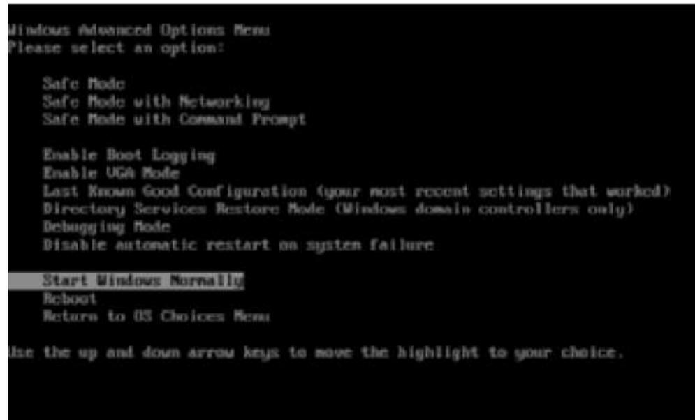
**Figure 6-43** Press the F8 key at startup to display the Windows XP Advanced Options menu
