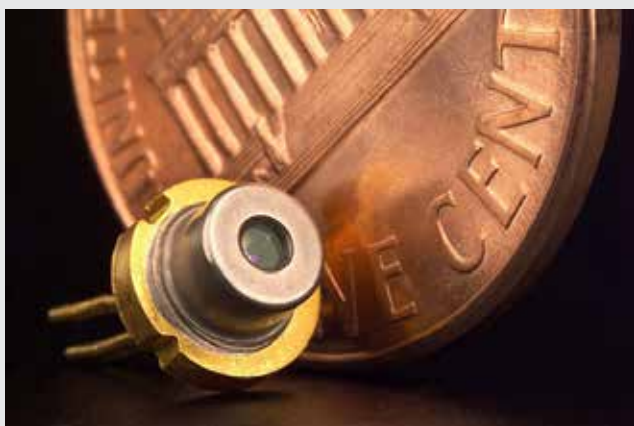
A laser diode, with a penny for scale.
