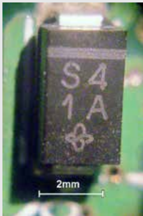
An electronic component that has been marked by a laser.
