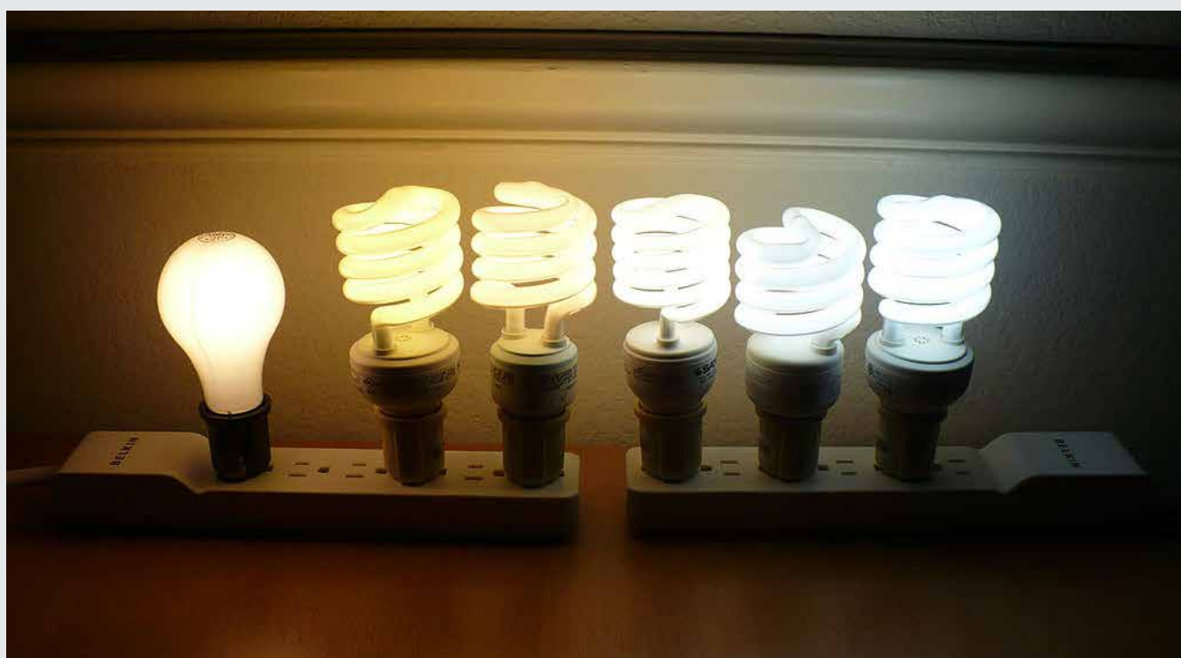
Comparison of an incandescent light bulb (left) and five CFL bulbs. They differ slightly in color due to different types of phosphor coating inside the tubes.
