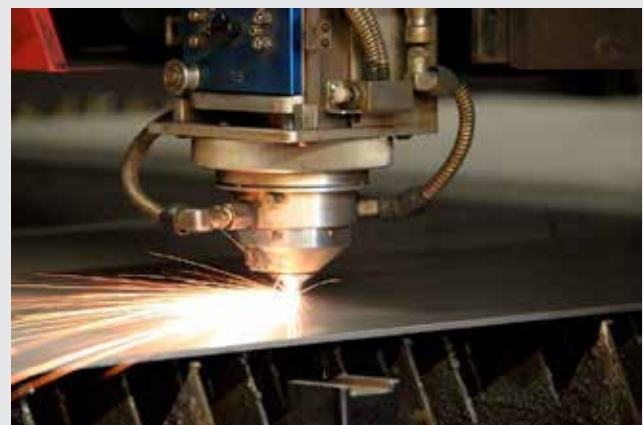
A four-kilowatt industrial laser cutting a sheet of metal.
