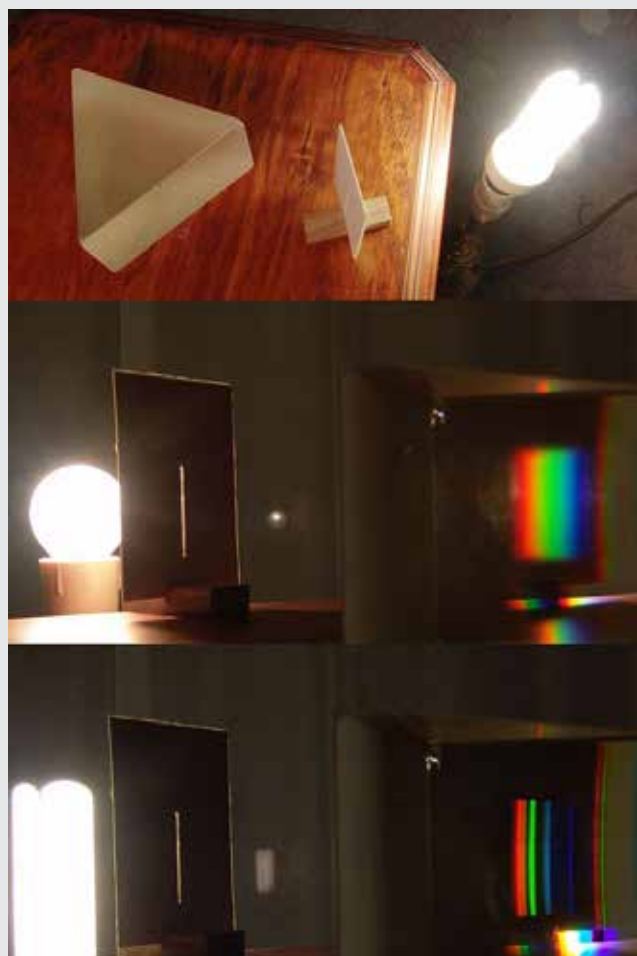
A basic spectroscopy apparatus using a prism and a narrow slit in cardboard (top). Notice the difference in spectral lines from an incandescent bulb (middle) and a fluorescent bulb (bottom).
