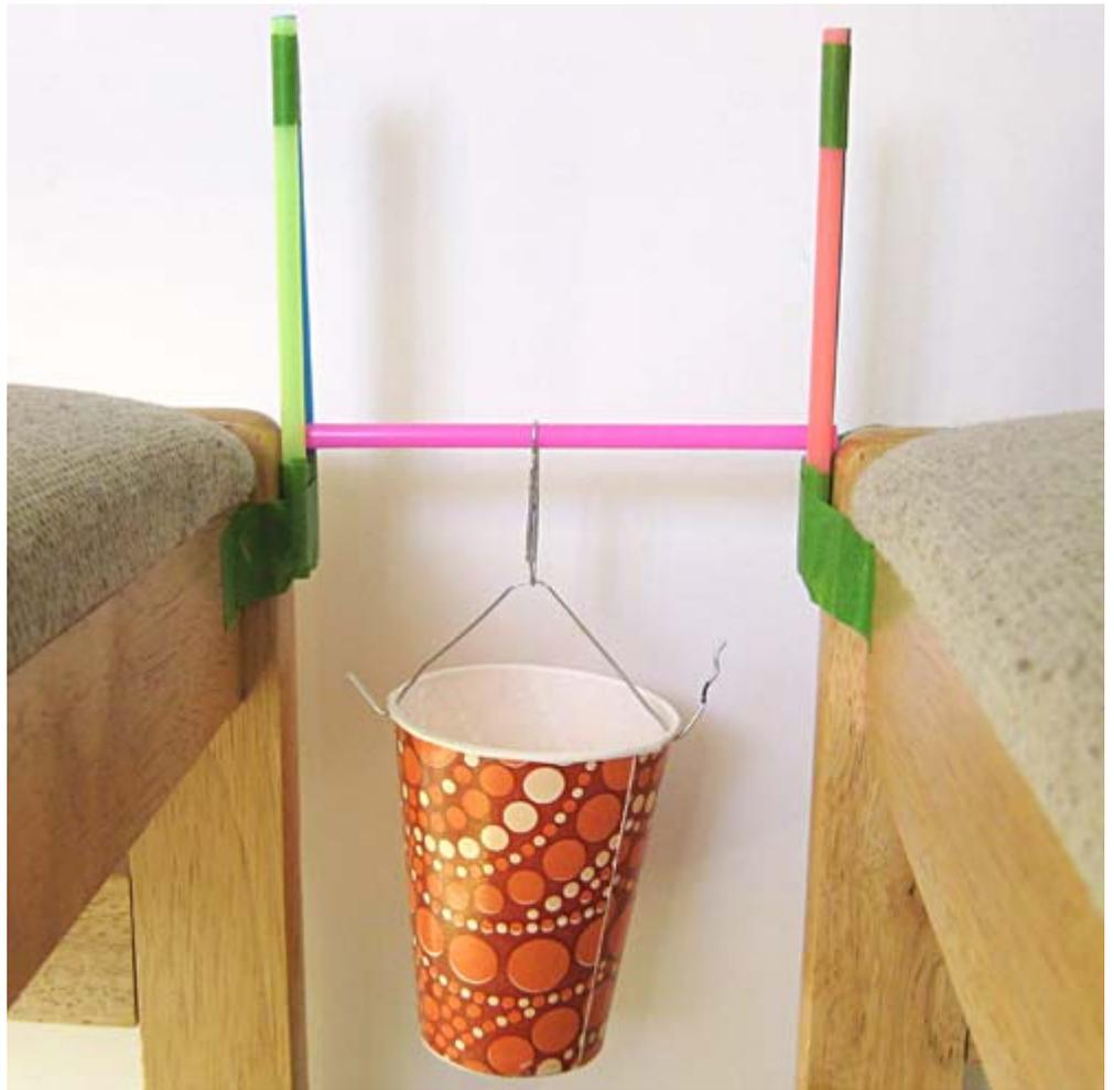
**Figure 10.** Attach the load tester (paper cup) to the bridge deck (the pink straw here) by using a second
