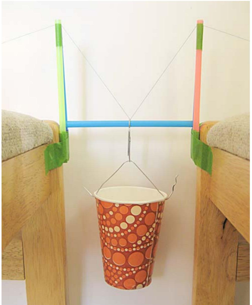
**Figure 13.** Attach the load tester (cup) to the bridge deck (the blue straw here) as you did be
