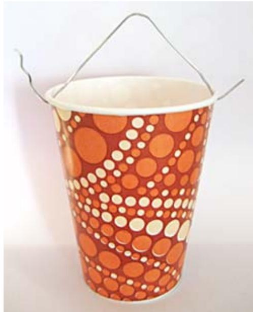
**Figure 9.** Make a load tester by bending a large paperclip into a V-shape and poking the ends into a paper cup, on opposite sides.
