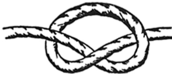
**Figure 3.** For each parachute, tie the ends of the strings together using an overhand knot, as sh
