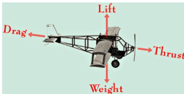
**Figure 1.** The aerodynamics of this airplane are due to the balance of four forces: lift, weight, thrust, and drag (image
