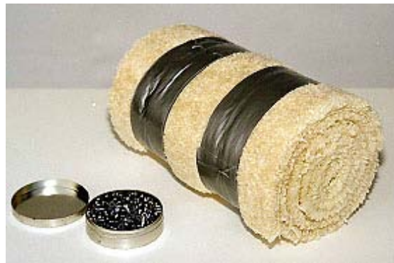
A suitable kneeling roll may be made by rolling a strip of carpet to form a roll. Tape the roll to keep it rolled tightly.
